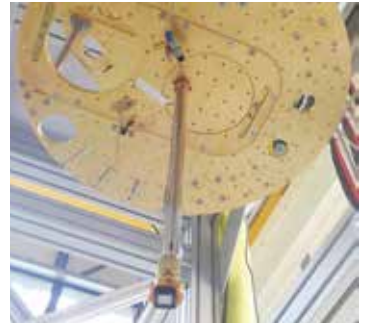
Paragraf cryogenic GHS mounted on an Oxford Instrument Proteox dilution refrigerator
