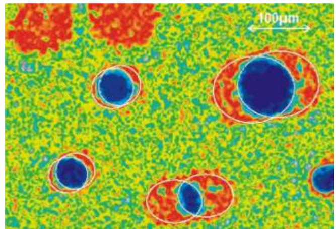
*The image shows particles imaged with dual laser illumination under a certain angle. The separation of the shades is a direct measure of the particles position within the viewing direction. Using this information the particle size and shape can be directly analyzed by the particles shades. Figure reprinted with permission of Universität der Bundeswehr, Munich.*
