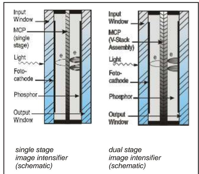
First the incoming photon releases an electron in the photocathode, second the electron is accelerated and amplified to an electron avalanche within the multi-channel plate (MCP), third the accelerated electrons are converted into photons by the phosphor screen.
