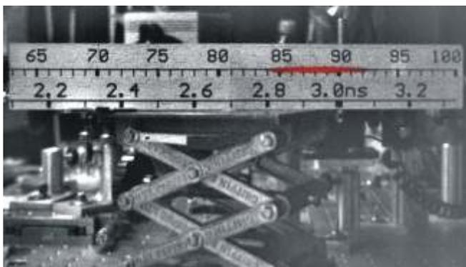
The image shows the distance a femtosecond laser pulse moved along a ruler while the shutter of the 4 Picos camera was open. This distance is a direct measure of the flat top, single shot gating time.
